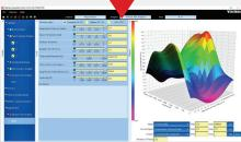
Start with a Thermal Desktop model, create a reducedorder model using Veritrek's Creation Tool, use the reduced-order model in Veritrek's Exploration Tool for rapid thermal analysis. To learn more, view the Veritrek software videos here.
